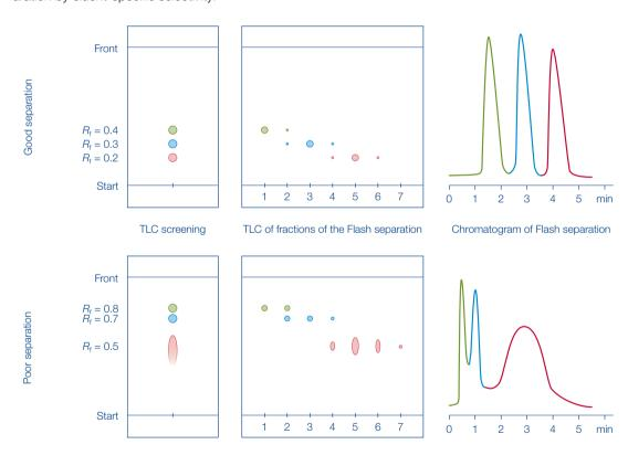
In flash chromatography, retention is expressed in column volumes (CV) which is the volume of solvent required to elute a non-retained compound or to keep it simpler, the dead volume. To isocratically elute the compound of interest 1/R<sub>f</sub> CV are required.
